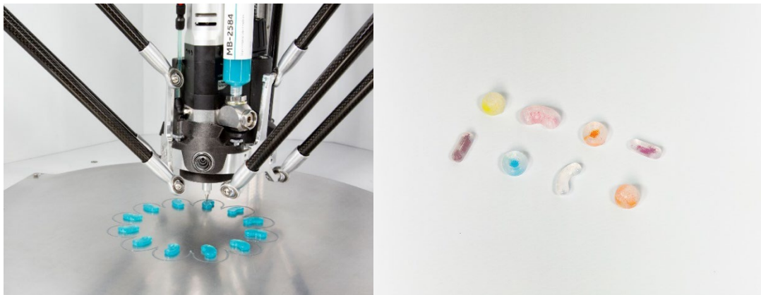
Medication 3D Printer: MED-U Modular and medications of various sizes and shapes
